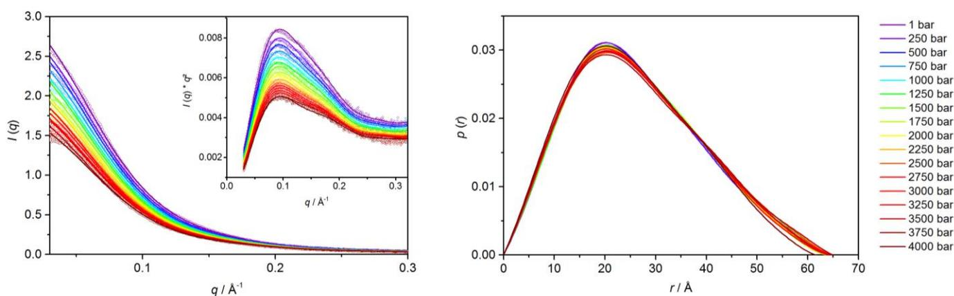
Figure 2: Pressure-dependent SAXS data of tRNA<sup>Phe</sup> at 20°C (3 wt% in 50 mM Tris-HCl buffer, pH 7.5, with 0.1 mM EDTA and 15 mM MgCl<sub>2</sub>). Intensity profiles at different pressures (left) with Kratky representation of the respective data (insert). Solid lines represent fits obtained by using the indirect Fourier-transformation method to calculate the pair-distance distribution functions (right).
