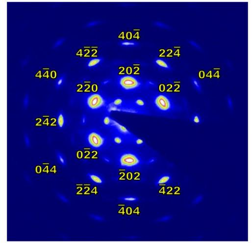
Fig. 1. Diffraction pattern for Co IOLS with thickness of 26 layers.
