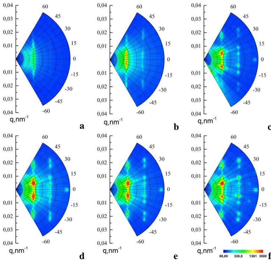
Fig. 2. Slice of the reciprocal space in plane  $(h0\bar{h})$  for the IOLS based on Co with number of layers of 0.5(a), 2(b), 7(c), 17(d), 20(e), 26(f)
