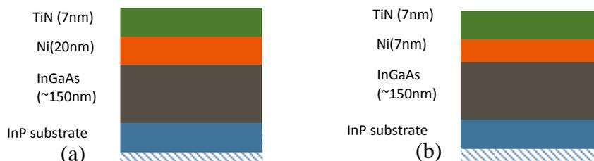
Figure 1. Scheme of the as-deposited stacks. (a) TiN/Ni(20 nm)/inGaAs/inP, (b) TiN/Ni(7nm)/inGaAs/inP
