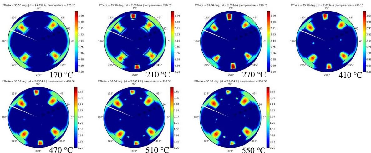
Figure 2. X-ray diffraction pole figures of Ni/InGaAs/InP sample (at different temperatures). The fixed angle was  $29.75^\circ$  corresponding to the intermetallic (101) reflection.
