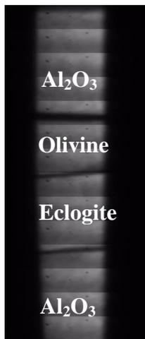
**Figure 2.** X-ray radiograph. Black lines are Re strain markers.  $\text{Al}_2\text{O}_3$  parts are pistons.
