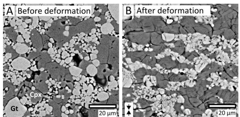
*Figure 1.* Eclogite microstructure before (A) and after (B) deformation. Note the striking formation of alternating garnet-cpx layers after compressive deformation. Some grains were plucked out from polishing.
