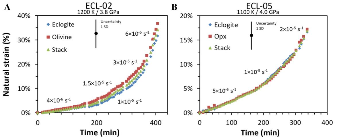
**Figure 3.** Natural (true) strain plotted against time for two experiments. The kinks in the curves are due to an increase in anvil displacement rate, leading to an increase in sample strain rates, as labelled. On the left (A), eclogite was placed in series with olivine. On the right (B), eclogite was placed in series with orthopyroxene. Systematic uncertainty in strain (from marker positions) is shown with 1 standard deviation. Opx – orthopyroxene.
