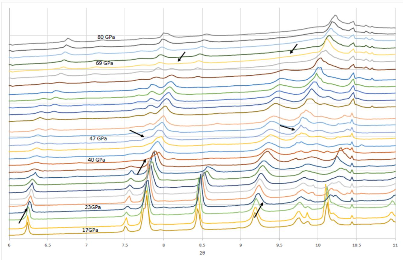
Fig.1 Evolution of the XRD pattern of AlFeO<sub>3</sub> at pressure range 17 – 80 GPa.
