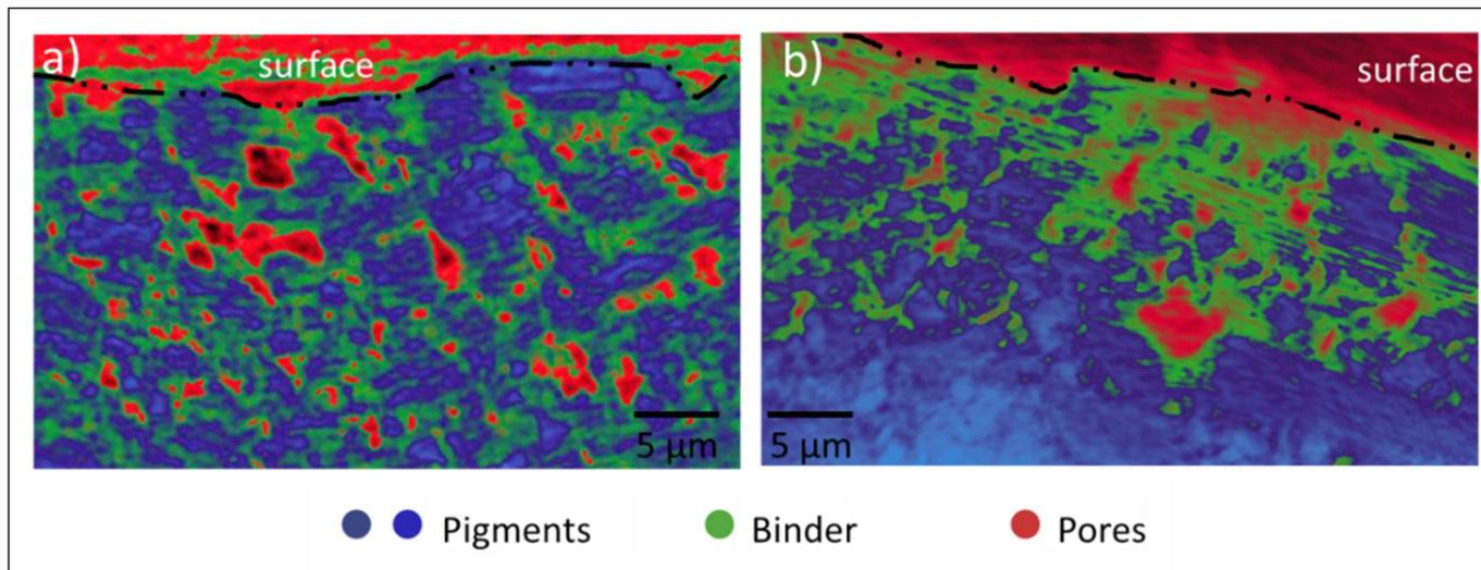
Figure 3: X-ray phase contrast nanotomography reconstructed images. a) altered; b) conserved paint micro-samples. Scale bars: 5 $\mu$ m.
