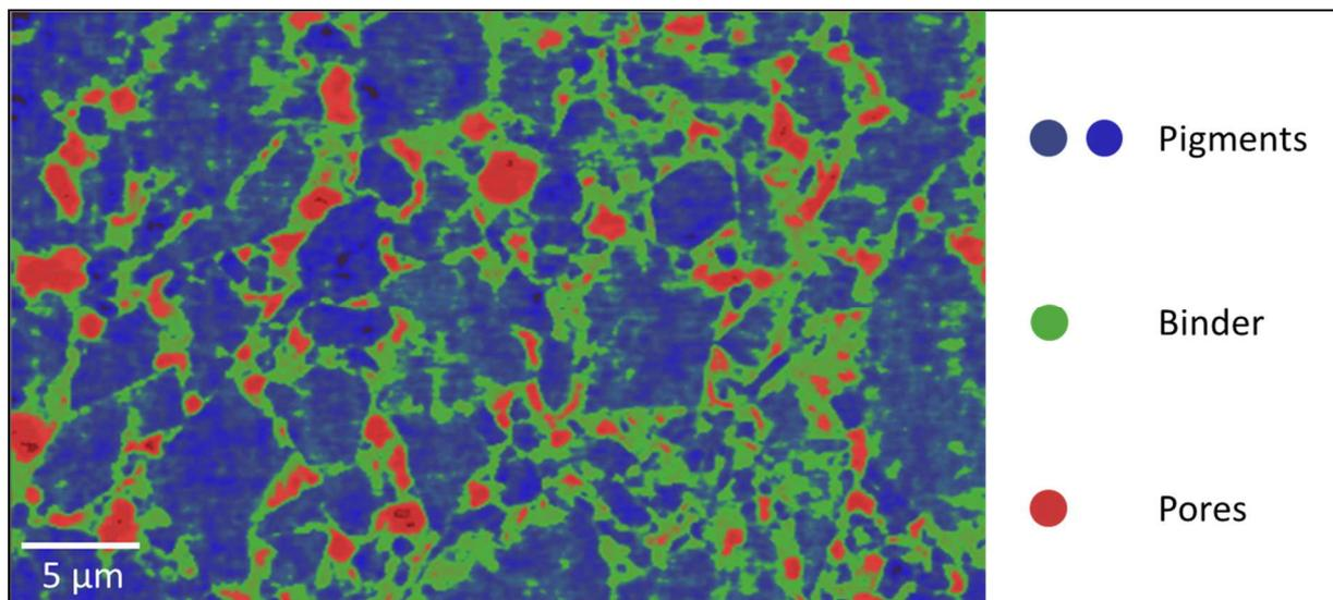
Figure 2: Detail of a reconstructed slice highlighting the presence of pores in the organic binder. Scale bar: 5 $\mu\text{m}$
