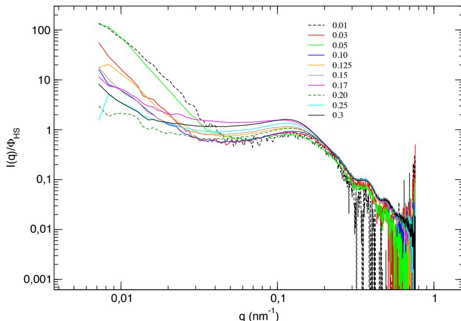
Figure 1. Scattered intensity vs.  $q$  ( $\text{nm}^{-1}$ ) normalized with particle concentration for the PEG grafted polystyrene colloidal particles dispersed in  $0.4 \text{ M Na}_2\text{CO}_3$  (aq) collected at the ID02 USAXS beamline. The legend show the particle volume fraction.
