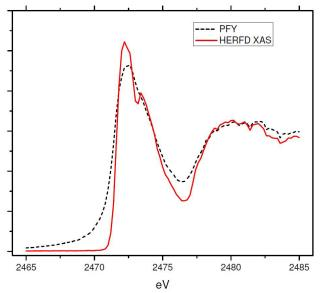
Figure 1: The S K-edge partial fluorescence yield (PFY) spectrum and high energy resolution fluorescence detected (HERFD-XAS) recorded on the  $S_8$  standard sample using the emission spectrometer.
