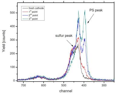
Figure 2: A sequence of first three resonant KL emission spectra of the LiS battery during the discharge process. Fixed excitation energy of 2470.3 eV was used corresponding to the PS peak in the HERFD spectra. Due to very high sensitivity the formation of PS is detected right from the start of the discharge process. The sulfate electrolyte peak is completely suppressed due to resonant excitation.
