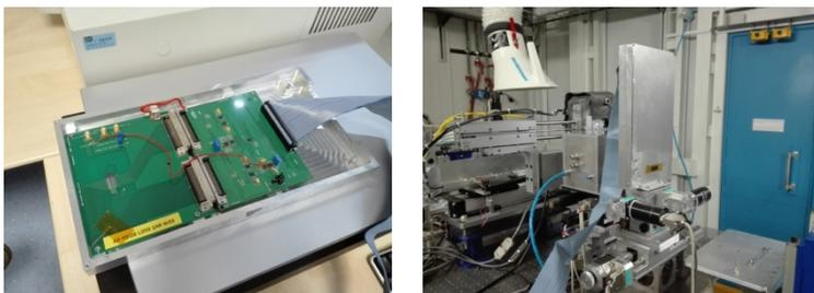
*Figure 1 – Left: the AFE readout daughterboard, connected to the sensor testboard, as mounted in the support frame. right: The complete support frame mounted on the ID 17 beamline.*
