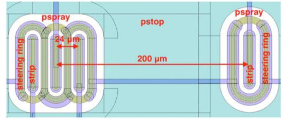
Figure 2: variable pitch sensor geometry
