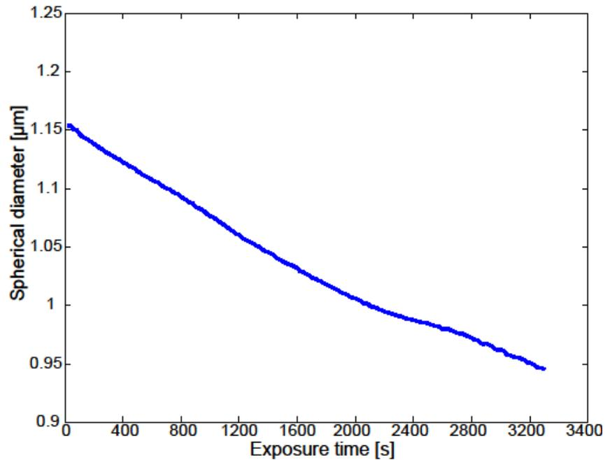
Figure 2: Diameter of pure polystyrene sphere as function of accumulated exposure time. The polymer is seen to suffer from radiation damage.
