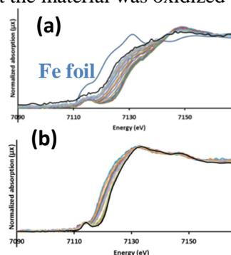
**Figure 1:** The Fe-K edge XANES spectrum up to 800°C of fresh 10-Mg-Fe-Al-O during (a) H<sub>2</sub>-reduction and (b) CO<sub>2</sub>-reoxidation
