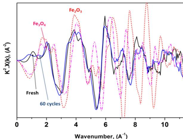
**Figure 5:** The k-space spectra of the fresh and cycled material, the latter after TPR and TPO, with references Fe<sub>2</sub>O<sub>3</sub> and Fe<sub>3</sub>O<sub>4</sub> measured at -196°C.
