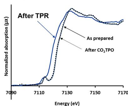
**Figure 2:** The room temperature XANES spectra of 10-Mg-Fe-Al-O in as prepared state, after H<sub>2</sub>-TPR and after CO<sub>2</sub>-TPO.
