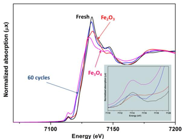
**Figure 4:** XANES of the fresh and cycled sample, the latter after TPR and TPO, with references Fe<sub>2</sub>O<sub>3</sub> and Fe<sub>3</sub>O<sub>4</sub>, and the inset showing pre-edge features of all these materials.
