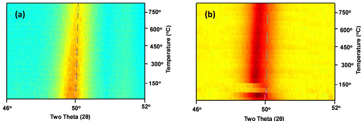
**Figure 3:** High resolution in situ XRD pattern of the most intense diffraction peak of 10-Mg-Fe-Al-O at Fe-K edge during (a) H<sub>2</sub>-reduction and (b) CO<sub>2</sub>-reoxidation
