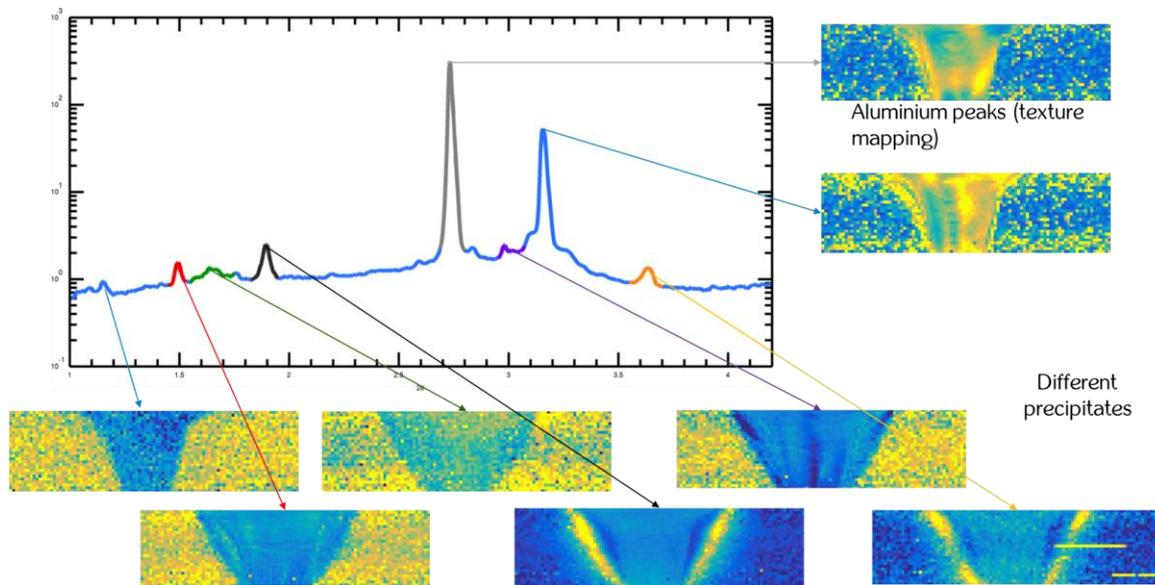
*Fig. 2 maps obtained on the various Bragg peaks in the WAXS signal. Indexation in underway.*
