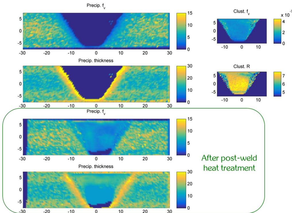
Fig. 1: microstructure mapping obtained on an Al-Li-Cu with and without post-weld heat treatment.
