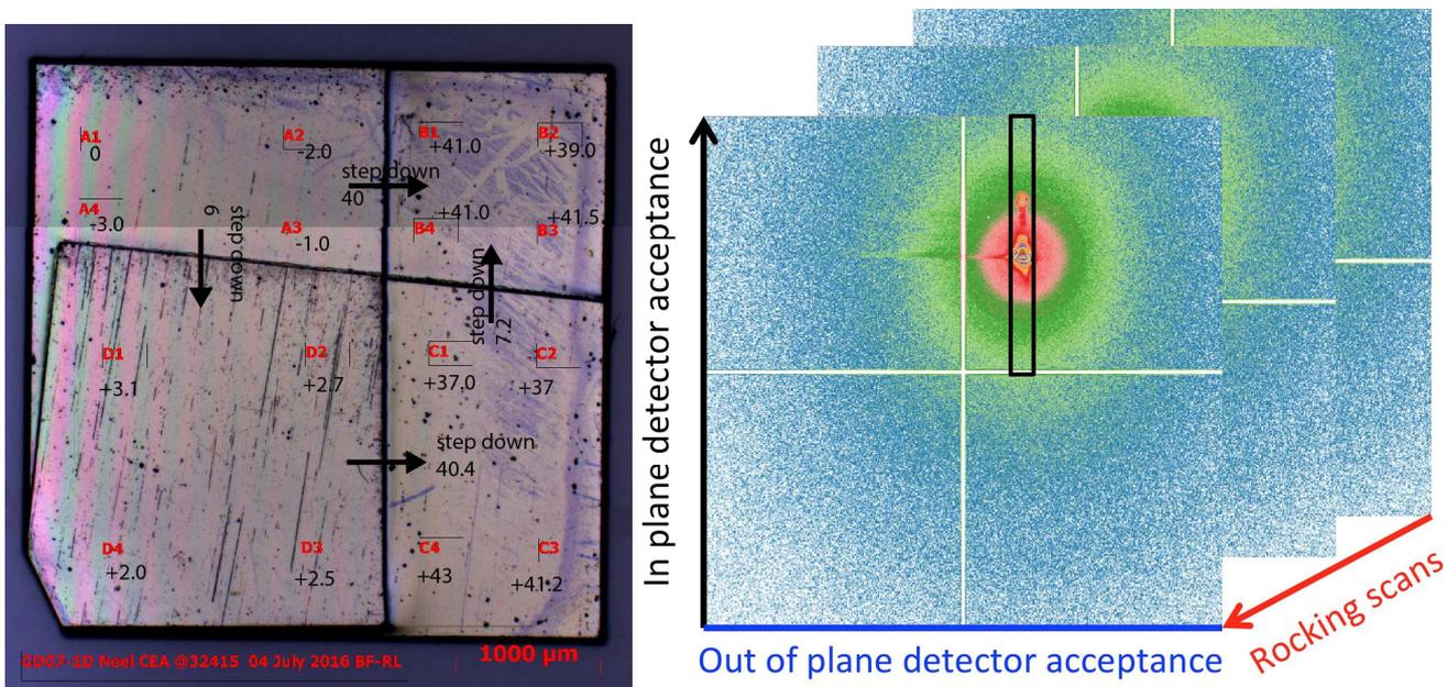
Fig. 1 : (left) optical microscopy image showing the four masked zones that underwent different etching processes and etch depths at CEA Saclay. (right) Stacks of 2D images acquired during a rocking scan that are used to reconstruct the in-plane intensity map, exploiting the large acceptance of the 2D pixel detector at ID01.
