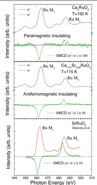
**Fig.1.** Top: Ru- $M_{2,3}$  XAS and XMCD spectra of Ca<sub>2</sub>RuO<sub>4</sub> (top panel), Ca<sub>1.81</sub>Sr<sub>0.09</sub>RuO<sub>4</sub> (middle panel) single crystals measured under applied field H = 8.5 T at ID32 beamline with circular polarized soft X-rays. Bottom panel: Ru- $M_{2,3}$  XAS and XMCD spectra of SrRuO<sub>3</sub> taken from [4].
