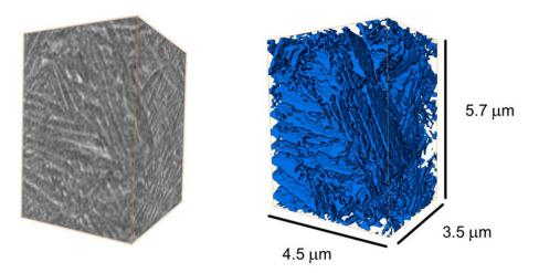
**Fig.1.** Illustrative perspective of an interconnected network of  $\beta$  matrix (in blue) segmented from its associated holographic X-ray computed tomography (HXCT) reconstruction (voxel size =  $(10 \text{ nm})^3$ . It corresponds to a representative volume of the microstructure of SLM-produced Ti-6Al-4V highly affected by the intrinsic heat treatment.
