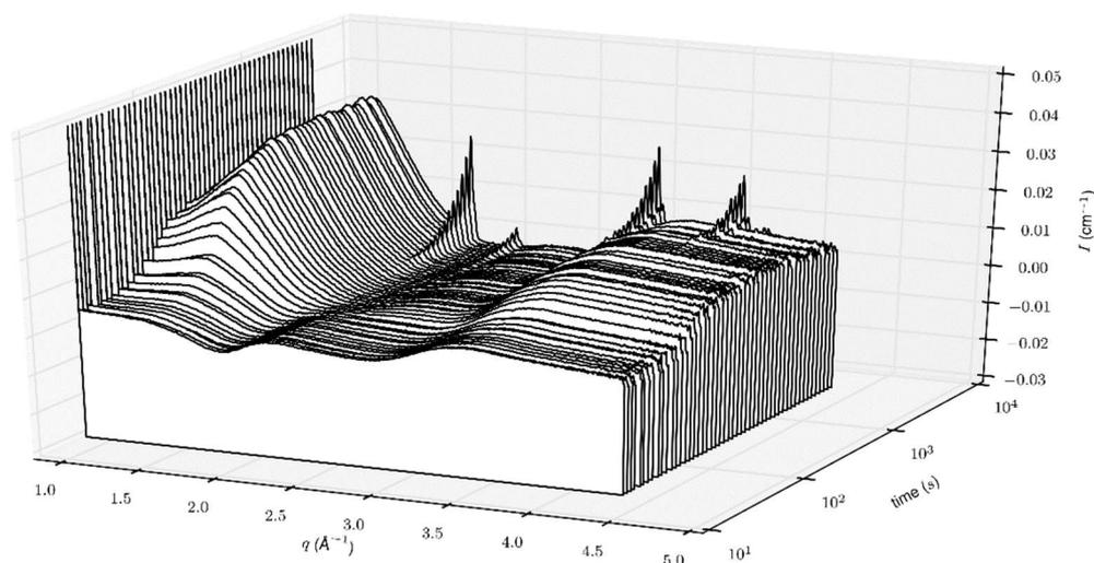
Figure 5. Selected WAXS patterns recorded during a  $\text{NaYF}_4:\text{Eu}$  synthesis with the peristaltic setup.
