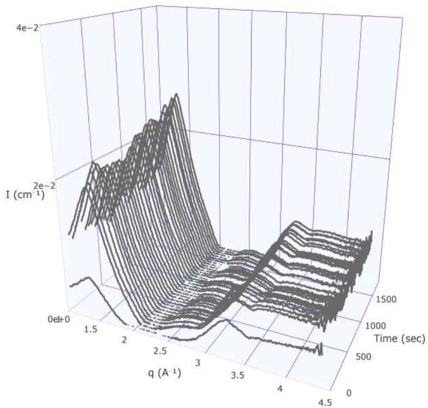
Figure 7. Selected WAXS patterns recorded during a  $\text{YF}_3\text{:Eu}$  synthesis with the peristaltic setup.
