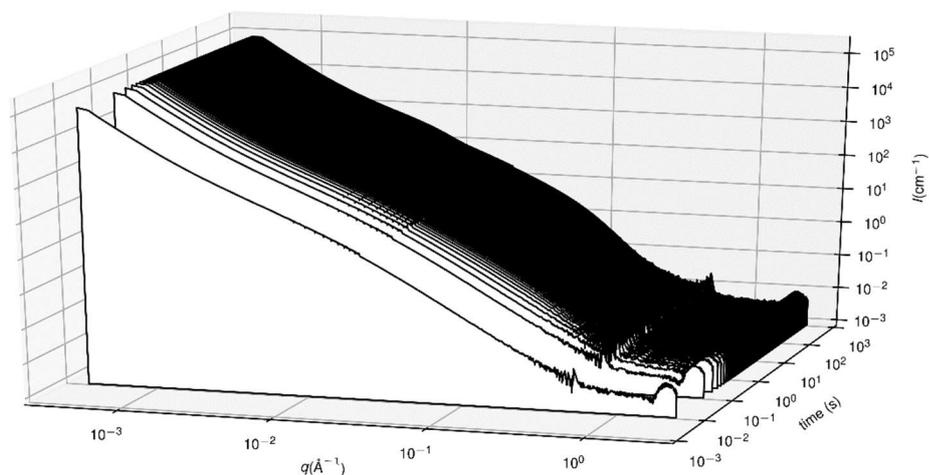
Figure 2. SAXS/WAXS patterns recorded during a NaYF<sub>4</sub>:Eu synthesis with the stopped-flow setup.
