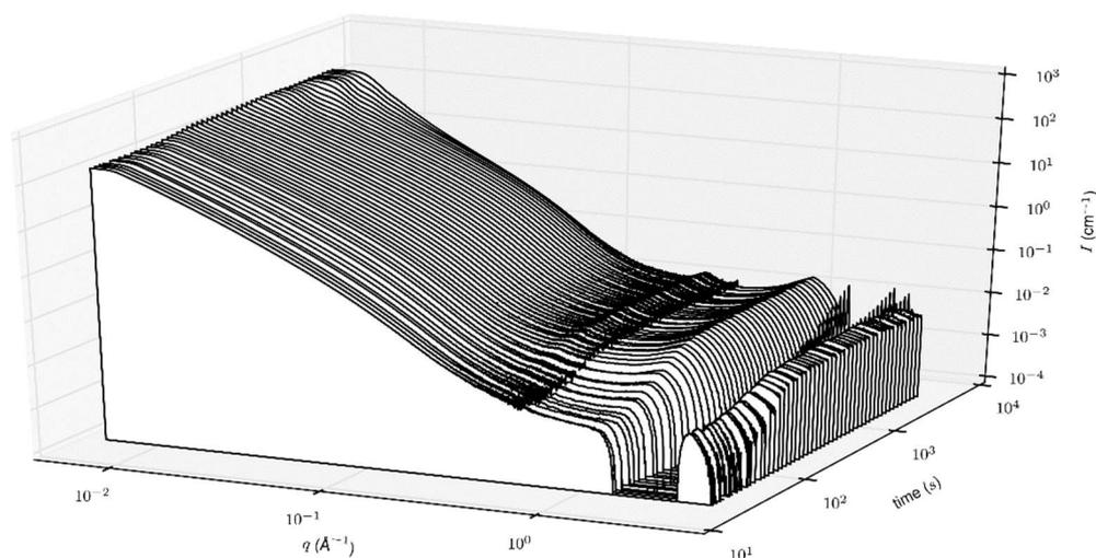
Figure 4. Selected SAXS/WAXS patterns recorded during a  $\text{NaYF}_4:\text{Eu}$  synthesis with the peristaltic setup.
