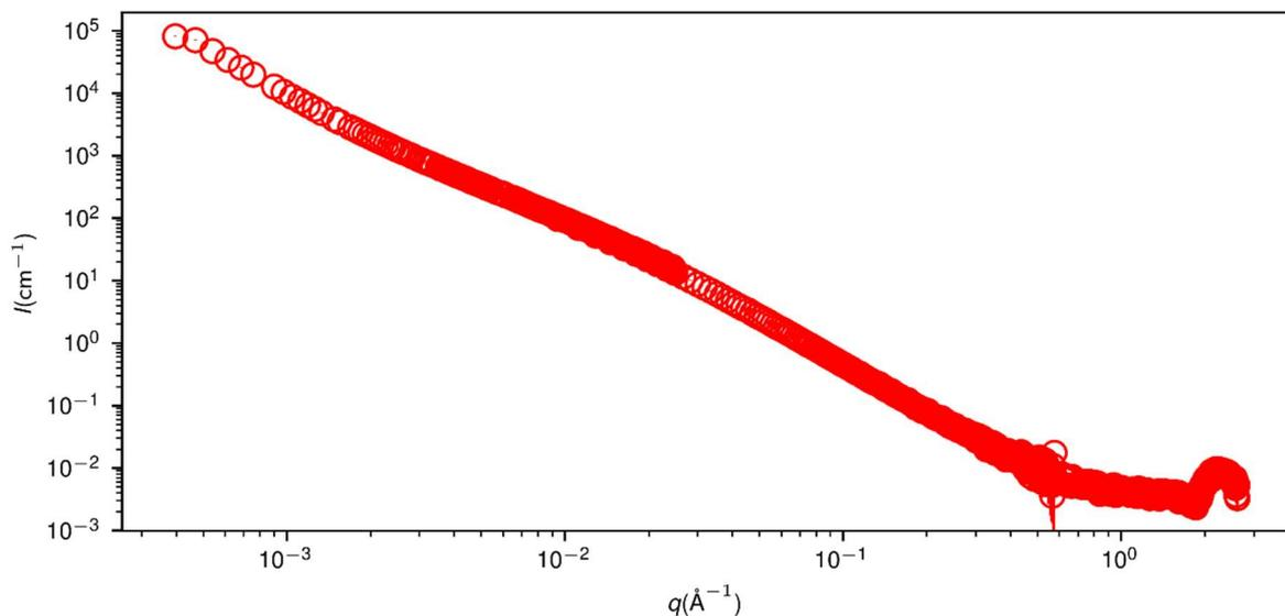
Figure 1. SAXS/WAXS pattern recorded for a NaYF<sub>4</sub>:Eu reaction, at reaction time  $t=6\text{ms}$ , using the stopped-flow setup in a lost-flow configuration.
