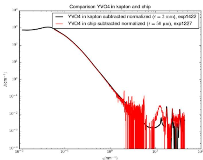
Figure 6. SAXS/WAXS signal of a dispersion of YVO<sub>4</sub>:Eu nanoparticles in water measured in a 2mm thick kapton capillary (black, 5ms acquisition time), and in a 50 $\mu\text{m}$  thick microfluidic channel (red, 10s acquisition time).
