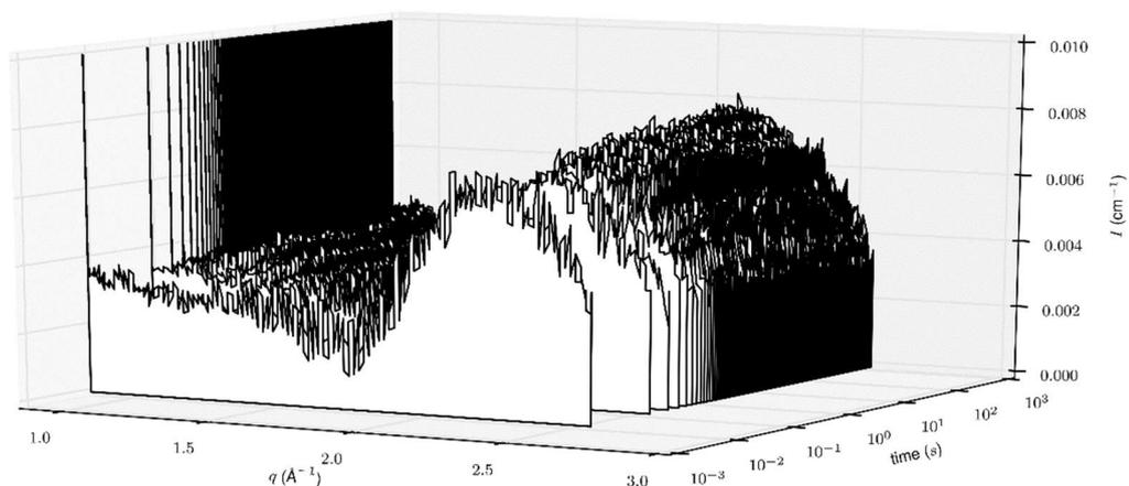
Figure 3. WAXS patterns recorded during a NaYF<sub>4</sub>:Eu synthesis with the stopped-flow setup.
