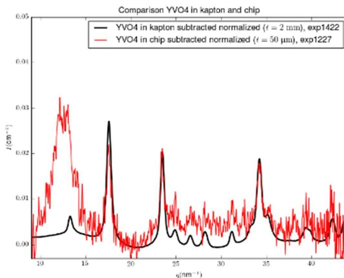
Figure 7. SAXS/WAXS signal of a dispersion of YVO<sub>4</sub>:Eu nanoparticles in water measured in a 2mm thickkapton capillary (black, 5ms acquisition time), and in a 50 $\mu\text{m}$  thick microfluidic channel (red, 10s acquisition time).
