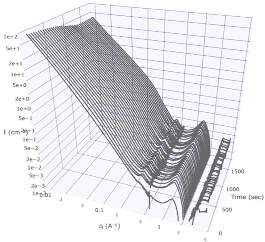
Figure 6. Selected SAXS/WAXS patterns recorded during a  $\text{YF}_3\text{:Eu}$  synthesis with the peristaltic setup.
