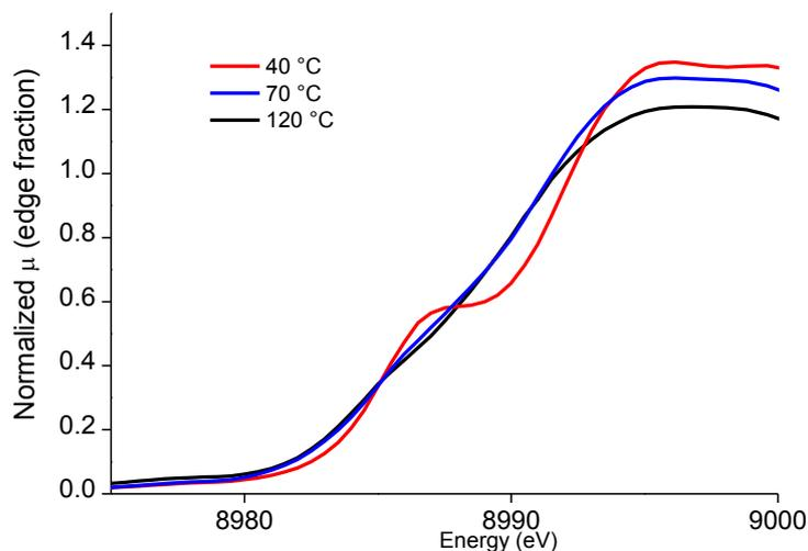
Figure 2. Absorption edges of Cu present in  $[\text{Cu}(\text{BuIm})_4][\text{Cl}]_2$  at different temperatures.
