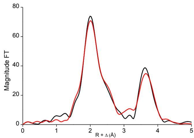
Figure 3a. EXAFS function (black) and model (red) of  $\text{Yb}(\text{NO}_3)_5^{2-}$  fitted in  $R$  space between 0 and 4.6 Å. Figure 3b. FT (black) and model (red) of  $\text{Yb}(\text{NO}_3)_5^{2-}$  fitted in  $R$  between 0 and 4.6 Å.
