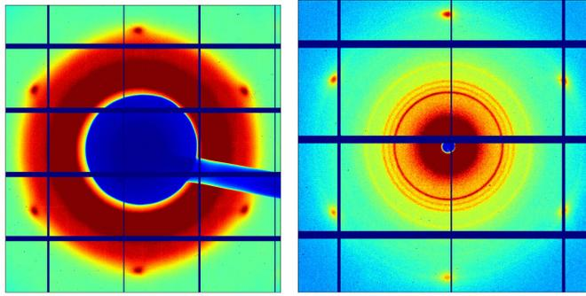
**Fig. 1:** Scattering from 0.6 mm Si(111) ( $E = 70$  keV, vertical incidence) with the beam passing through 4.0 mm (left) and 0.5 mm (right) of electrolyte. Intensities are normalised to the Si 1st order peaks.
