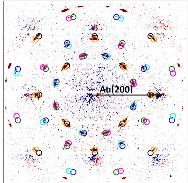
**Fig. 2:** Scattering ( $E = 70$  keV, vertical incidence) from 30 ML Bi(012) electrodeposited on (a) Au(111) and (b) Au(100), displayed as intensity difference between scattering from the bare electrode and after deposition. Bi(012) peaks marked in the same colour belong (per image) to the same rotational domain. Some peaks are obscured by detector tile edges.
