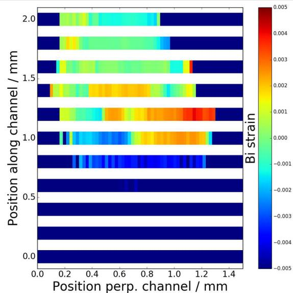
**Fig. 3:** TSD surface microdiffraction studies of a Bi(012) film on Au(100), demonstrating the extraction of structural properties. (a) Intensity (logarithmic scale) of an in-plane Bi(01-4) peak, corresponding with film thickness (b) Strain calculated from shifts in peak position. The electrolyte flow was along the up-down direction.
