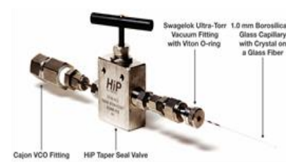
Figure 2- Designed in-situ powder cell
