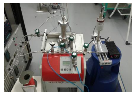
Figure 1- The gas dosing manifold designed for connection of the sample cell to vacuum or different gas sources
