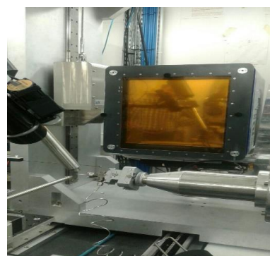
Figure 4- Picture of in-situ cell on the beam (at BM01)
