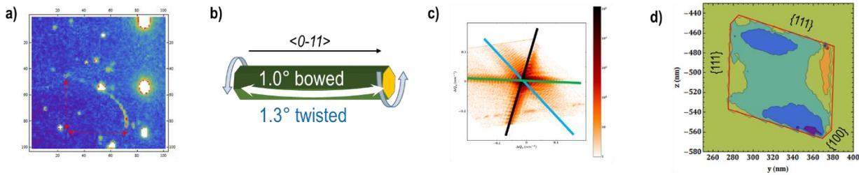
Figure 2. a) Sum of {311} peak along the wire measured in BM32 b) schematic of as-manipulated nanowire understood by the micro-Laue analysis c) {311} Bragg peak measured in ID01 before straining d) 2D reconstruction of the wire
