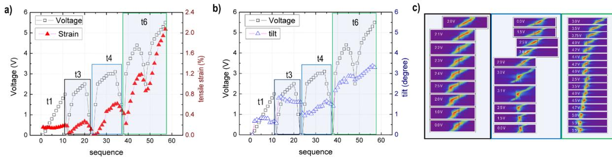
Figure 3. Applied voltage (actuation) is overlaid with a)  $\langle 110 \rangle$  tensile strain and b) angular movement of {311} peak in reciprocal space. c) Qz sum of the {311} Bragg peak during the tensile tests
