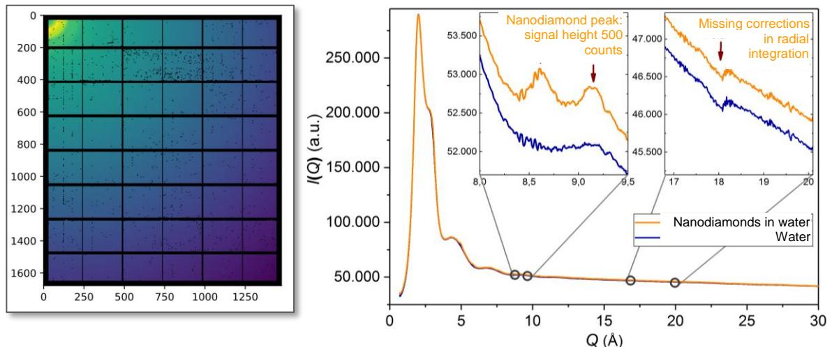
The integration of the detector, in particular with asymmetric primary beam positions, resulted in kinks in the data as shown in the figure to the right, where the signal height of the nanodiamonds is compared to the “kink” signal from the insufficient data integration. In order to analyze such challenging dispersions, a proper correction for dead and masked areas is utmost important.
