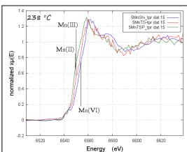
Figure 2. Normalized XANES spectra showing a different reduction degree of the indicated samples sunder 10 % H<sub>2</sub> at 238 °C. The Mn content is 5% in weight.
