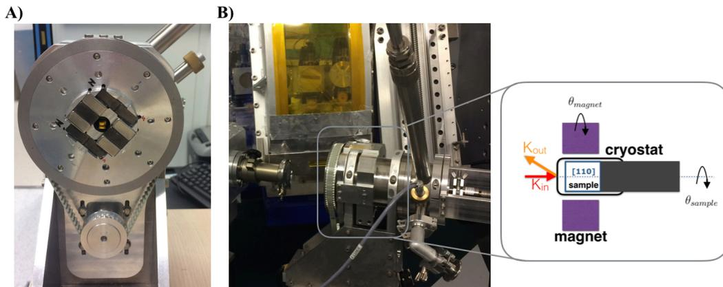
**Figure 1:** Setup developed at ID20. **A)** Front view showing the magnets arrangement surrounding the cryostat. The magnetic field is ~0.5T in the centre. **B)** Side view showing the scattering geometry used. A cartoon on the right illustrates possible rotations in the setup ( $\theta_{\text{sample}}$  and  $\theta_{\text{magnet}}$  are the rotations of the sample and the magnet).
