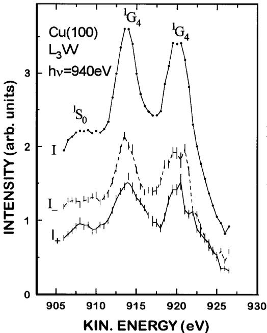
Fig. 1: Distorted spin resolved  $L_3VV$  Auger spectrum measured at  $h\nu=940\text{eV}$  at Cu(1 00).  $I_+$  and  $I_-$  give the partial electron intensity with spin parallel and antiparallel to the photon spin, respectively.
