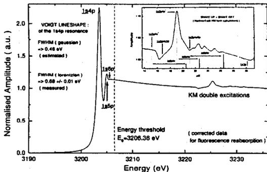
Fig. 1 XANES spectrum of Ar gas with KM multielectron excitations
