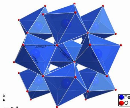
Fig. 1. Crystal structure of cubic  $\text{FeO}_2$  as refined from single-crystal diffraction data collected at 58(1) GPa. Shortest O–O distance is 2.137(2) Å characteristic for  $\text{HP-PdF}_2$ -type structure.
