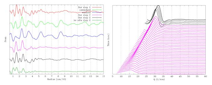
Fig1. a) PDFs extracted from raw data without corrections (left), b) in-situ addition of 2-propanol as ligand. Depicted are difference data sets with respect to file 1 (start of the synthesis) in a time frame of 1.5 hours (right).
