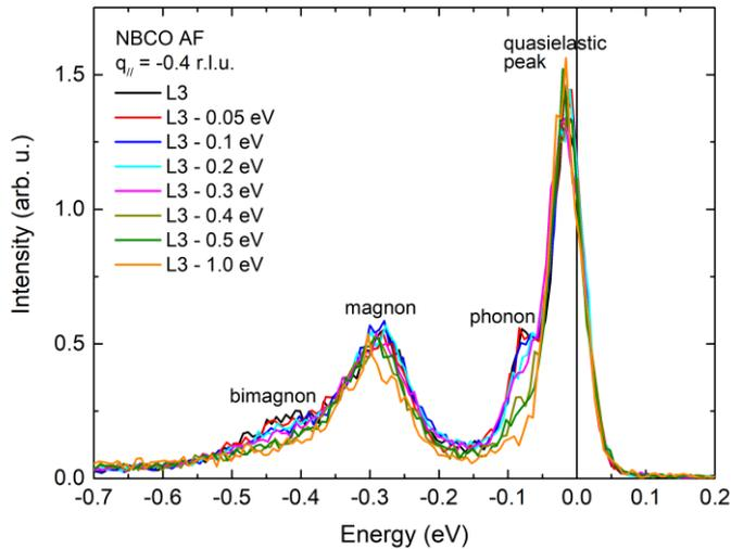
**Figure 1** RIXS spectra of NBCO measured at different incident photon energies below the Cu  $L_3$  edge absorption peak. The spectra are normalized to the spectral weight of the  $dd$  excitations (not shown).
