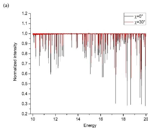
**Fig. 5.** Two EXAFS spectra of the diamond plate with two different  $\chi$  angles.
