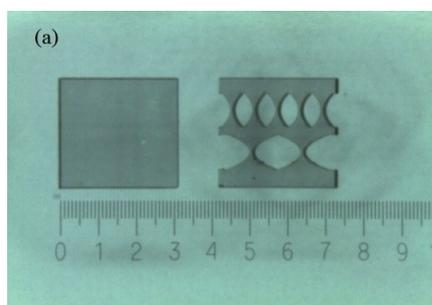
**Fig. 4.** Optical micrograph of two diamond plates used for experiment and described in this report.
