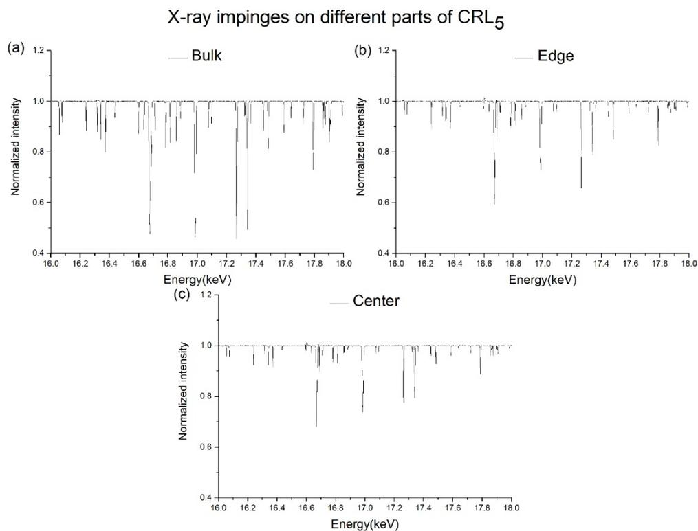
**Fig. 8** Various location of the incident beam with respect to CRL<sub>5</sub> affects EXAFS spectrums.
