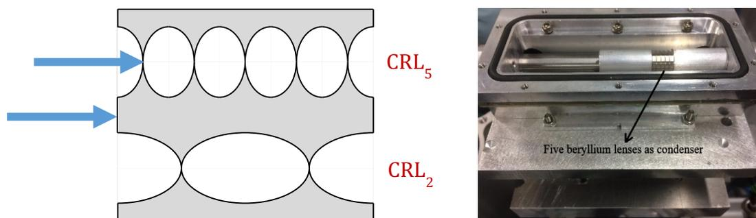
**Fig. 6.** a) Schematic drawing of diamond lenses with two arrays of compound lenses and bulky material in between. b) The condenser CRL.
