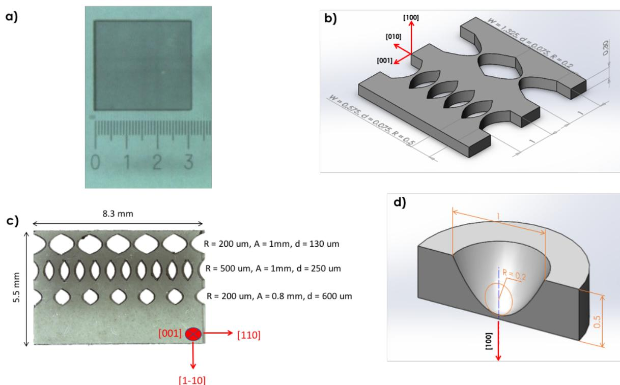
**Figure 1.** Four types of diamond plates used for the experiment – no profiling (a), one-dimensional CRLs made from slightly different diamond materials (b-c) and two-dimensional lens (d). Red arrows show crystallographic directions. Dimensions are in mm.
