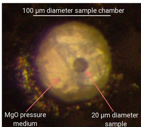
*Typical sample preparation. Polycrystalline olivine, shaped into disks of 30  $\mu\text{m}$  diameter and 15  $\mu\text{m}$  thickness, with a 100 nm coating of platinum on both sides, loaded in MgO pressure medium inside a 100  $\mu\text{m}$  diameter hole in a rhenium gasket.*
