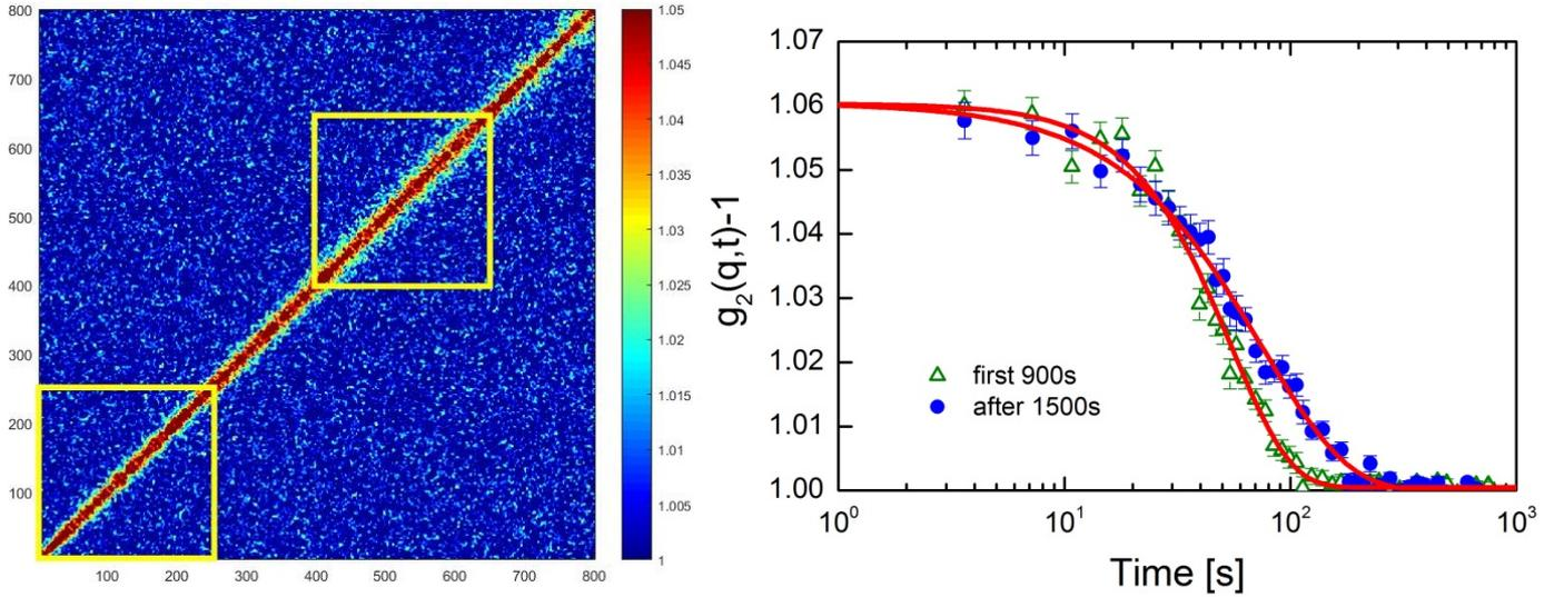
*Figure 1:* (left) Two-time correlation function measured at room temperature at the maximum structure factor  $S(Q)$  on the  $x=5$  CAS sample. Left to right in frame number ( $\Delta t = 3.6$  s). The yellow squares indicate the frames used to calculate the correlation curves plotted in Figure 2.
