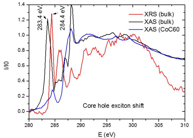
FIG. 2. Comparison of the K-edge in  $C_{60}$  films obtained via XAS and XRS. When a thin film of  $C_{60}$  is interfaced with a metal film,  $\pi$  resonances are suppressed and a shoulder feature emerges close to the Fermi energy due to filling of hybrid interface states. This is the key feature which indicates coupling to the metal substrate.
