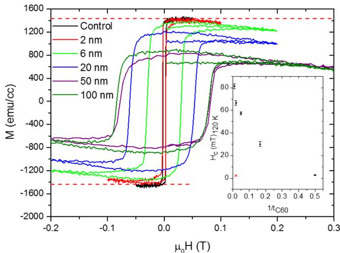
FIG. 1. Hysteresis loops in  $\text{CoC}_{60}$  bilayers obtained via VSM. The target was to observe films in the range of 200 - 20 nm, where the most significant changes in magnetic properties occur. The red dotted line marks the  $M_{sat}$  of the control sample in which a layer of alumina separates the  $C_{60}$  from the metal layer.
