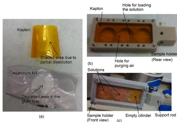
**Figure 1.** Sample preparation. (a) Damage to kapton® and glue on the rear of an Al foil due to exposition to  $\text{CH}_2\text{Cl}_2$ . (b) Sample holder, rear view. (c) Sample holder, front view.
