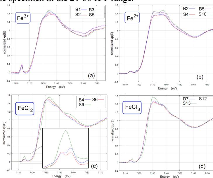
**Figure 2.** Comparison of relevant spectral features in representative samples here examined. (a) Hematin Fe(III) solutions. (b) Phthalocyanine Fe(II) solutions. (c)  $\text{FeCl}_2$  solutions. (d)  $\text{FeCl}_3$  solutions.
