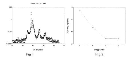
There is however, a presently unexplained asymmetry in the FWHM of the transverse scans as a function of satellite order around the 002 Au/Fe peak (Fig 2). The data show that there is a very small range of mosaic around the 001 direction in the high GMR samples grown on cubic MgO [2]. The samples on sapphire substrates show predominantly 111 orientation with much larger rocking curve widths and absence of clear satellites in the longitudinal scans.
