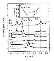
Diffraction from the cobalt clusters. The peaks that move when L changes indicate that the clusters have triangular section. The lateral faces are close to the (110) planes of hcp cobal
