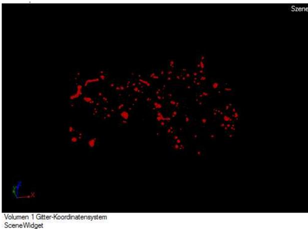
**Fig. 2** CMSX-4 after heat treatment, the porosity increases, the dendritic structure is not visible
