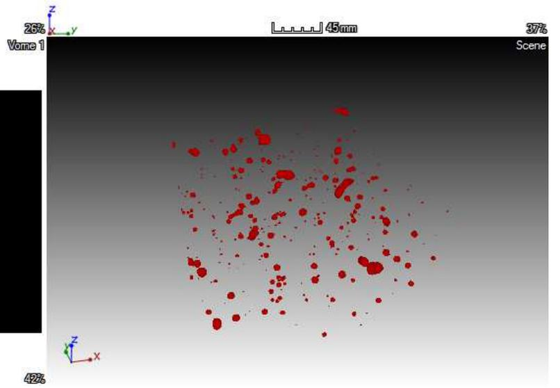
**Fig. 6** Porosity in deformed CMSX-4, creep condition:  $T=1100^{\circ}\text{C}$ ,  $\sigma=105\text{MPa}$ ,  $t_1=100\text{h}$
