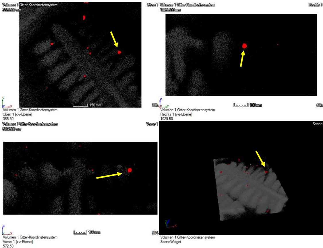
**Fig. 1** CMSX-4, initial as-cast state, different views of a selected void in the dendritic structure
