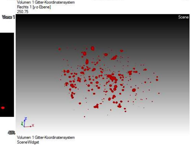
**Fig. 7** Porosity in deformed CMSX-4, creep condition:  $T=1100^{\circ}\text{C}$ ,  $\sigma=105\text{MPa}$ ,  $t_2=600\text{h}$
