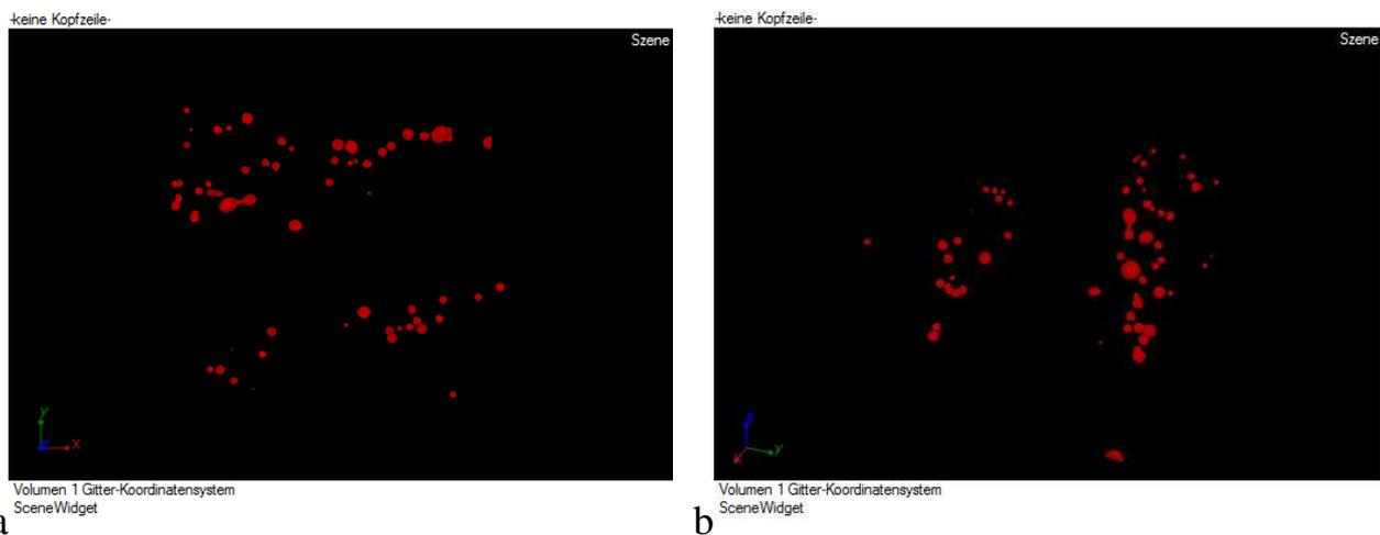
**Fig. 4** CMSX-10, as-cast and homogenized at 1350°C for 128h, voids arranged in rows (a+b: different views)
