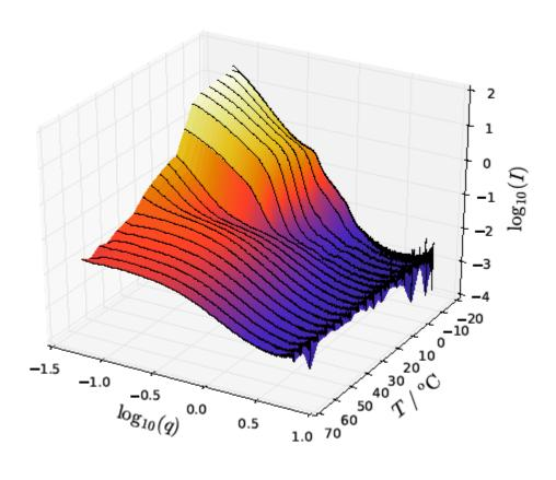
Fig 1. Background-subtracted scattering data for one of the copolymers in pure ethanol as a function of temperature.
