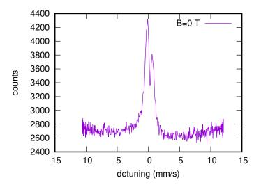
Figure 1: Data set of reflectivity as a function of energy detuning for the cavity structure Pt 3/C  $18.5/^{57}$ Fe-SS 0.6/ C 22.5/ Pt 15 and incidence angle driving the third cavity mode. Despite zero external magnetic field, the resonance shows a clear electric quadrupole splitting.
