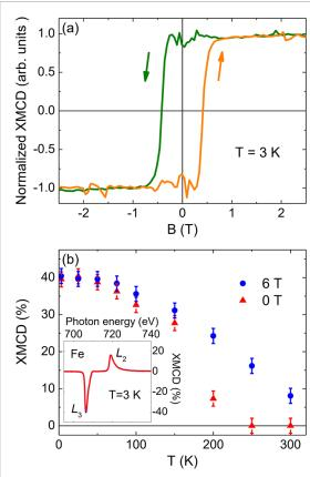
**Figure 4.** (a) Hysteresis loop recorded at the Fe  $L_3$  edge for a Te-capped,  $\sim$ 20 nm thick FGT film on graphene/SiC(0001) at 3 K. The XMCD signal is normalized to its value in saturation. (b) Temperature dependence of the Fe  $L_3$  XMCD maximum in saturation (6 T, blue circles) and remanence (red triangles). Inset: XMCD signal, expressed in percentage of the average XAS, recorded at 3 K under an out-of-plane magnetic field of 6 T (blue) and at remanence (red).
