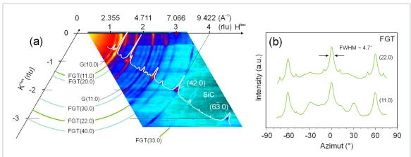
**Figure 2.** (a) GID in-plane reciprocal space map of a Te-capped 10 nm thick FGT on graphene/SiC(0001), reflecting the azimuthal dependence of various in-plane lattice parameters. The white line shows a linear scan along the SiC[ $2\overline{1}$ .0] direction. (b) Two azimuthal intensity profiles intersecting the maxima caused by the FGT lattice.
