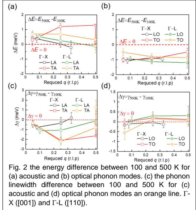
Fig. 2 the energy difference between 100 and 500 K for (a) acoustic and (b) optical phonon modes. (c) the phonon linewidth difference between 100 and 500 K for (c) acoustic and (d) optical phonon modes an orange line.  $\Gamma$ -X ([001]) and  $\Gamma$ -L ([110]).
