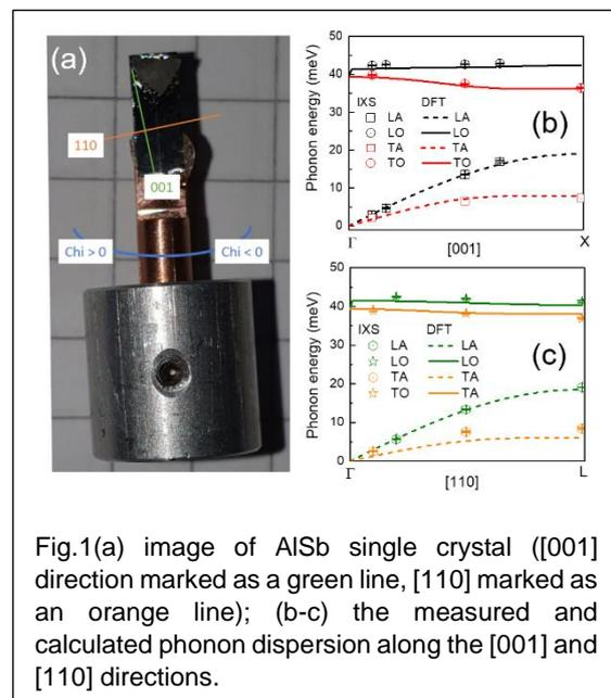
Fig.1(a) image of AlSb single crystal ([001] direction marked as a green line, [110] marked as an orange line); (b-c) the measured and calculated phonon dispersion along the [001] and [110] directions.
